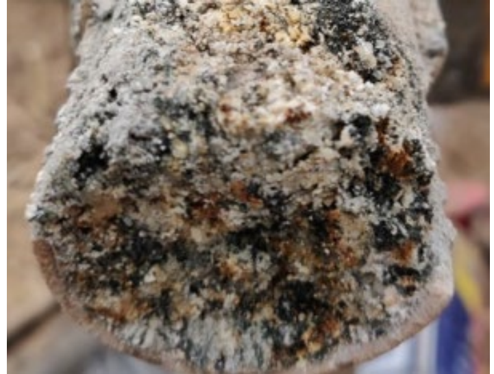
Figure 4-5. Unit 2 Weathered Tonalite
